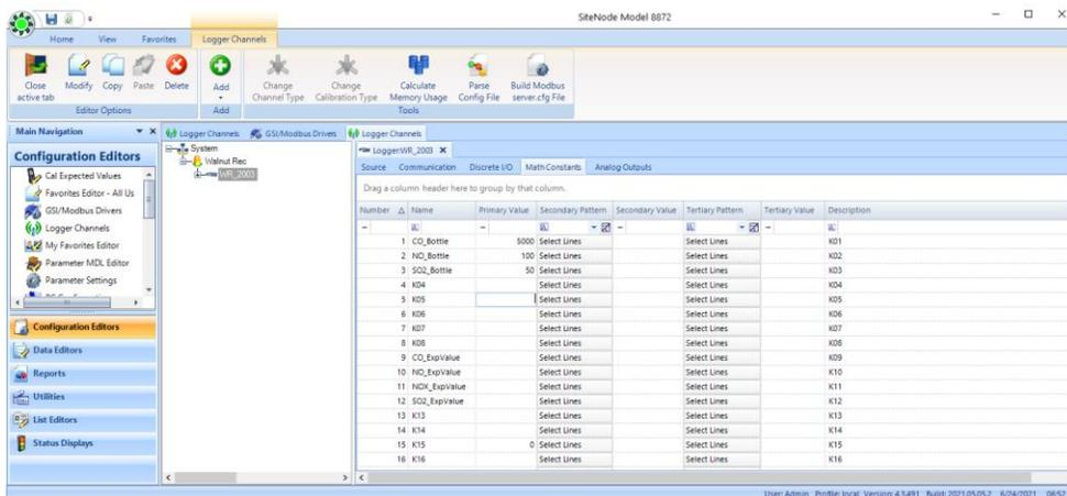
Then, we need to create channels (Modbus, GSI, etc) to log the CAL\_FLOW and DIL\_FLOW measurements in the calibrator.
