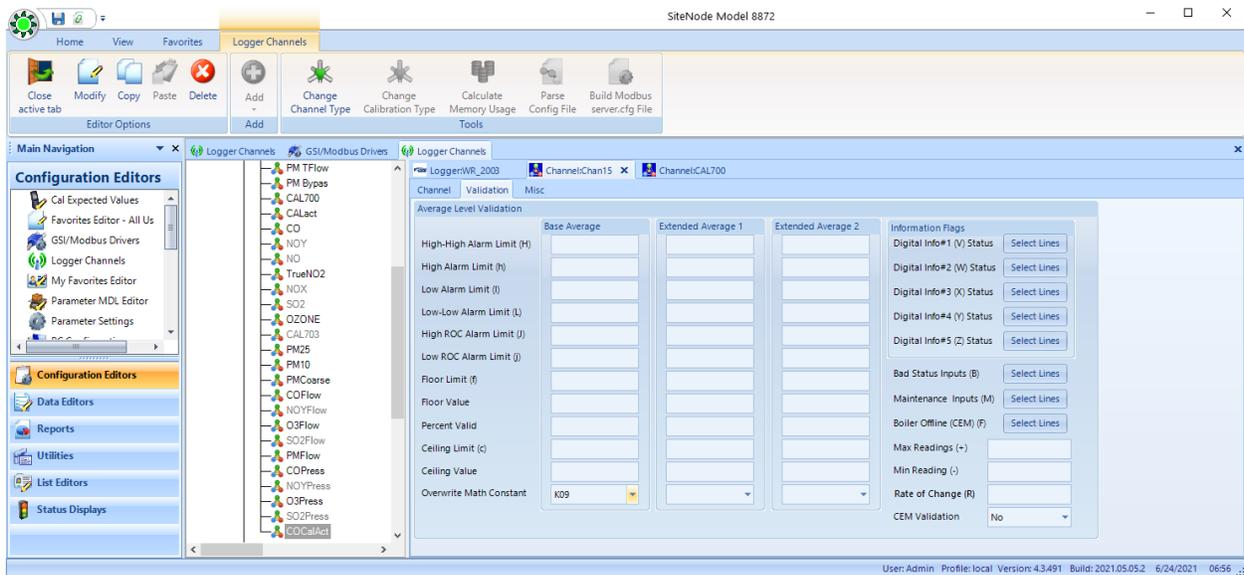
So, to do NO, CO, and SO2, we will need 6 math constants, 2 flow channels, and 3 calculated value channels. One set could potentially be eliminated as the 'default' gas in the calibrator and using the GASCONC channel.
