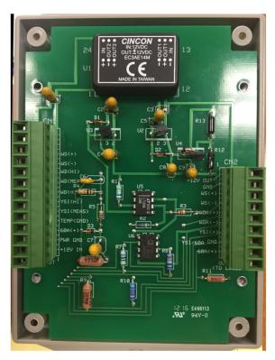
When you open the case, you will see CN1 on your left, which represent the sensor inputs, and CN2 on your right, which represents the outputs to go to the Model 8872 Status / Voltage Inputs. The bottom left side also has the input for a 12VDC power supply to power the device. Not all the inputs and outputs must be used (e.g., the device may be used only for wind speed, or a temperature input, and the others may be left open). The pairing and use of inputs and outputs is as follows:
